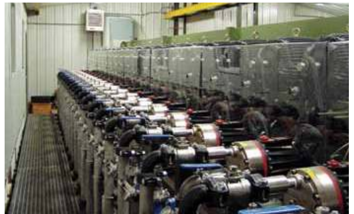
Hydra-Cell pumping shear-sensitive polymers for enhanced oil recovery.
